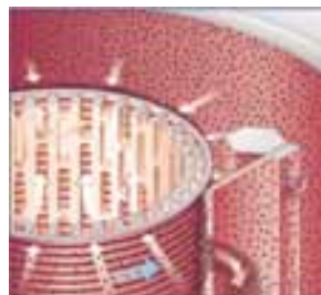
| Segment cleaning by internal pressure
