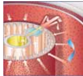
The principle of pulsating segment cleaning by external pressure surges
