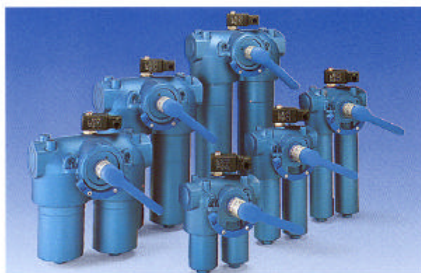
Pi 370 Rated flow 50 - 450 Connection G 1 - SAE 1 1/2" Nominal pressure (bar) 200/250
