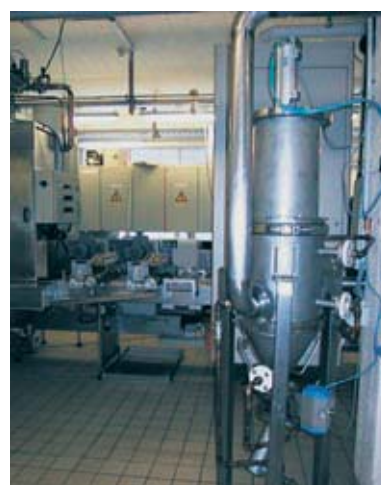
Automatic Metal Edge filter with an axial scraper cleaning device for chocolate
