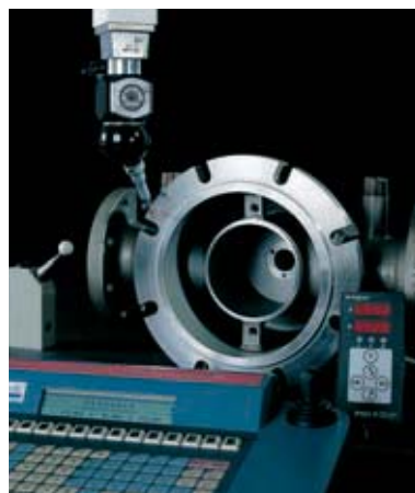
Quality assurance on a three-dimensional measuring machine
