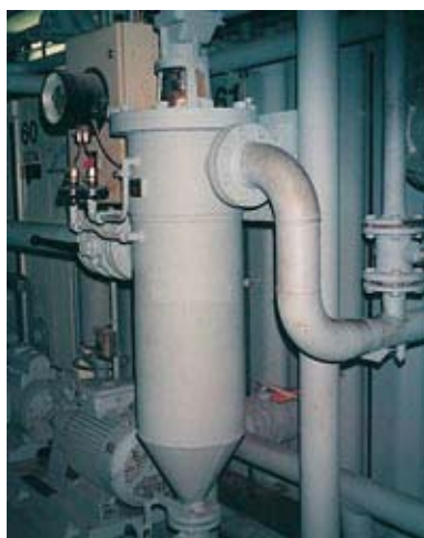
Automatic Metal Edge filter with a radial scraper cleaning device for isocyanate (a component of PU)
