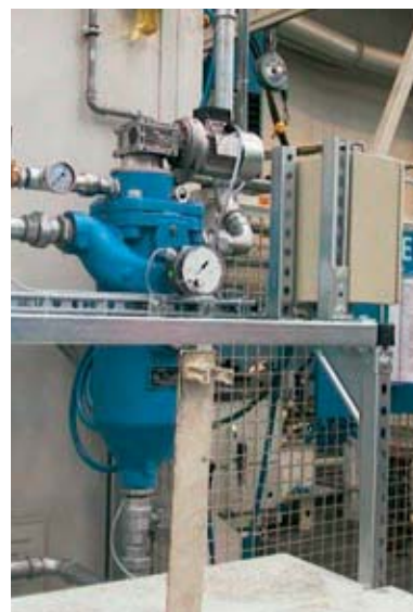
Automatic filter with external compressed air cleaning for cooling lubricant
