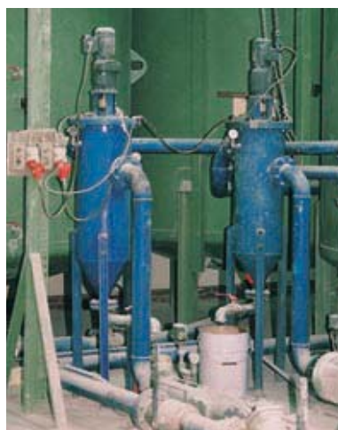
Automatic Metal Edge filter with a radial scraper cleaning device for adhesives
