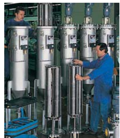
Final assembly of the Metal Edge filters
