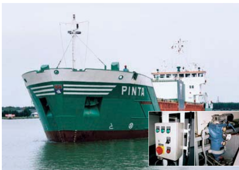
Automatic filter with internal pressure cleaning in marine application for engine oil
