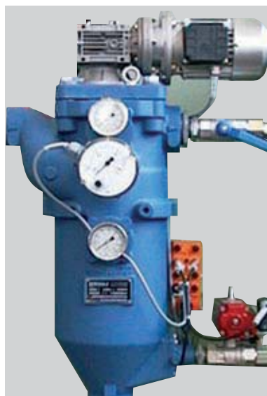
Automatic filter with internal pressure cleaning for cooling lubricant
